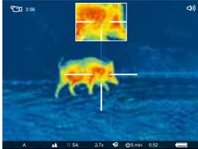
Picture-in-Picture improves accuracy by providing a magnified image of the reticle area at the top of the display. With only 1/10 of the display area reserved for PiP, the field of view remains virtually unobstructed for simultaneous PiP and FOV viewing.
