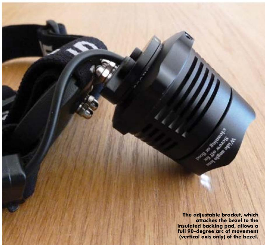
The adjustable bracket, which attaches the bezel to the insulated backing pad, allows a full 90-degree arc of movement (vertical axis only) of the bezel.
